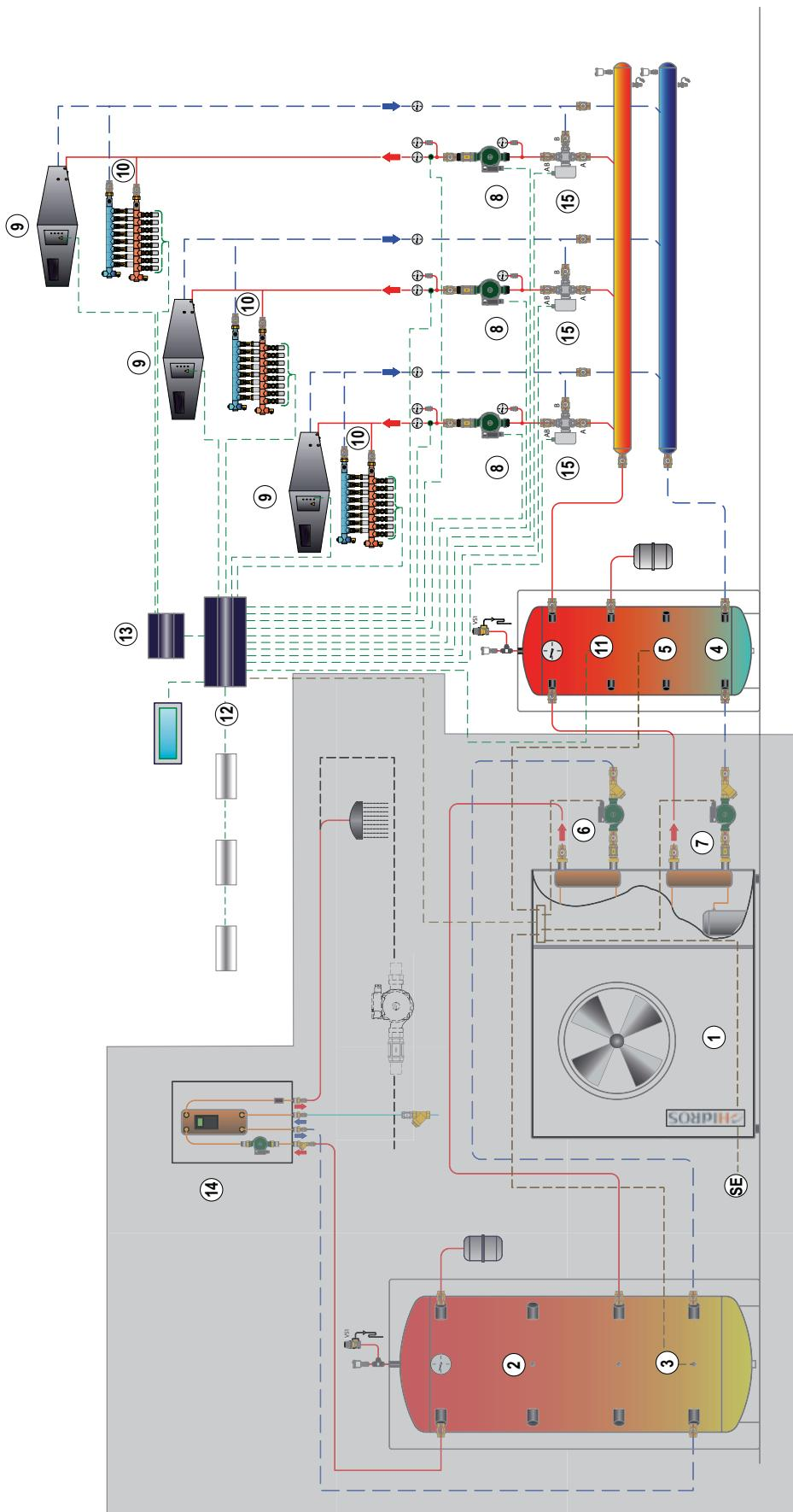
Installation of a control system for an air to water heat pump model L7T(LZA)/SW6 version, with DHW circuit priority, equipped with weather -compensated ambient sensor.
