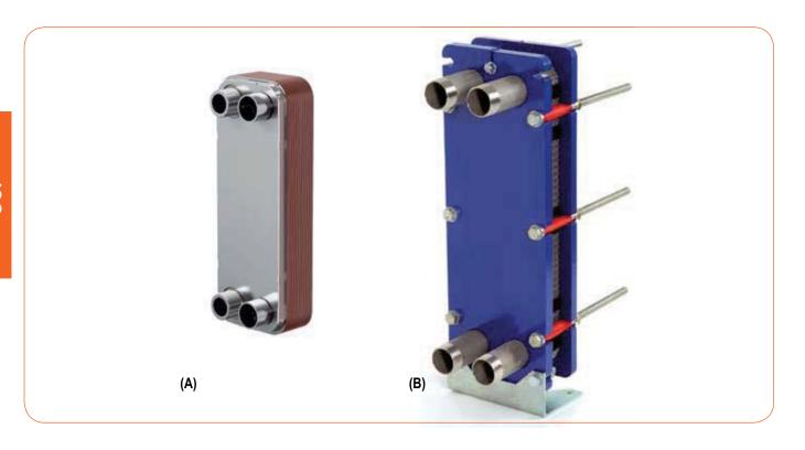
The SCP plate eschangers are designed for the production of the domestic hot water in combination with heat pump systems. The heat exchanger up to 20 Kw of heating capacity are brazed type, not inspectionable (picture A) while the bigger sizes are inspectionable and fixed with bolts and gaskets.
